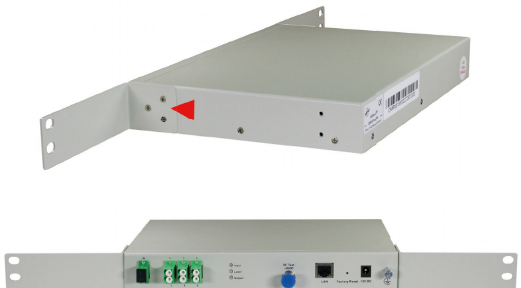
Figure 1c: mounting the OAMPc in a 19 inch cabinet
