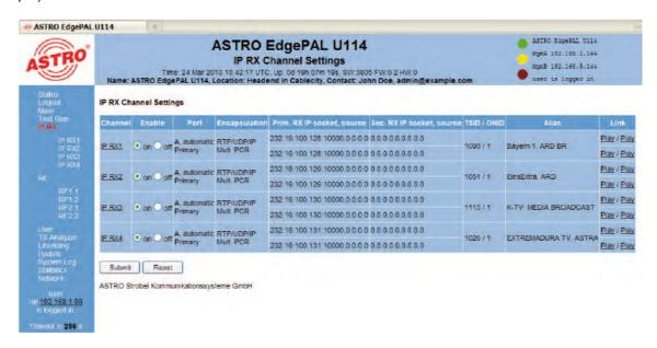
Figure 10: Overview of the IP input configuration
