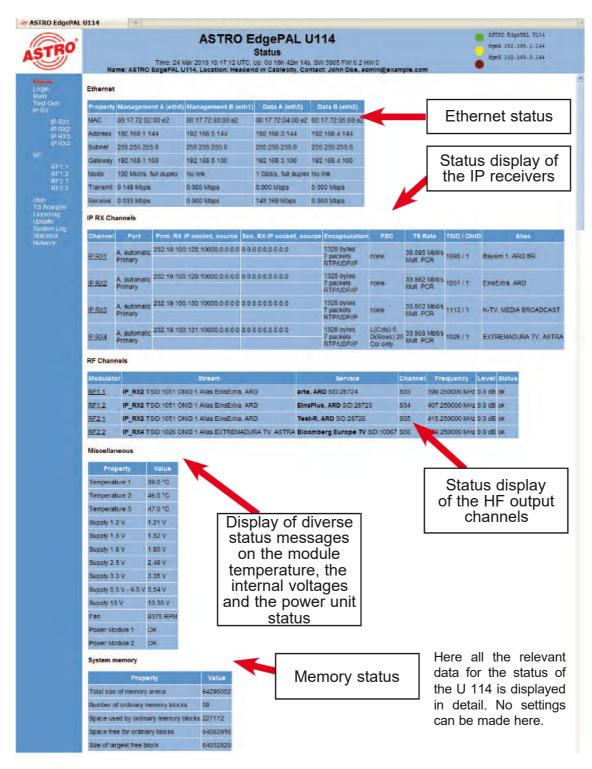
Figure 3: Status display in the "Status" submenu
