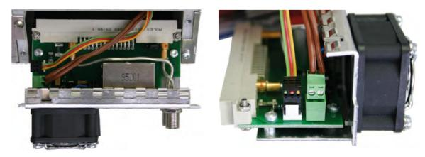
Figure 3: Connecting the voltage supply and signal lines
