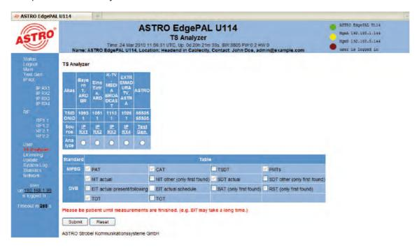
Figure 19: Transport Stream (TS) Analyzer view
