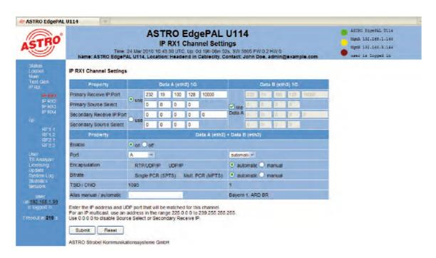
Figure 11: Detailed settings of the IP receiver
