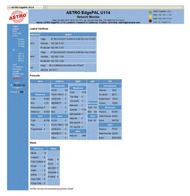
Figure 26: Example view of the network properties in the "Network Monitor" submenu
