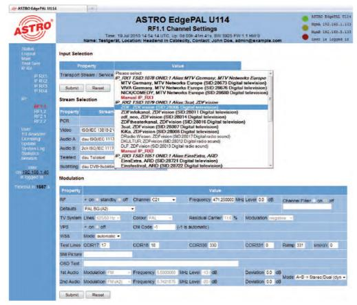
Figure 15: Output channel setting
