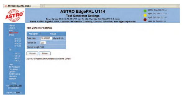
Figure 9: Test generator settings
