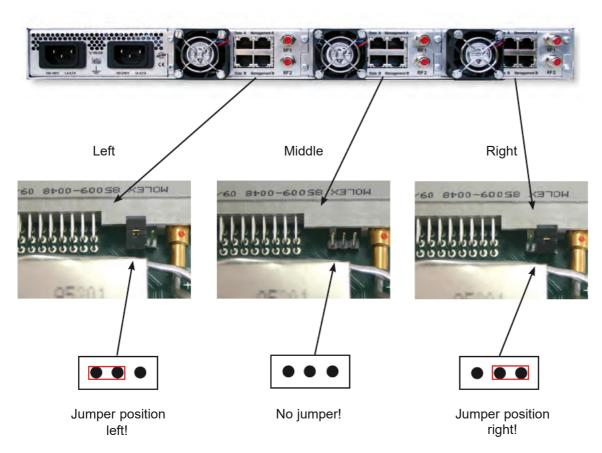
Figure 1: Coding the backplane using the jumper
